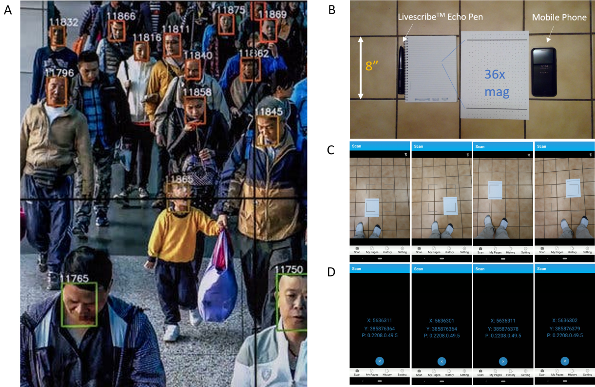
Figure 3. Precise geolocating of the masses versus precise geolocating for the masses. A. Face tracking in China (photo adapted from Ref. (19)). B. Visual positioning technology. Left-to-right: a pen that can stream its location on lightly patterned paper, within the diameter of its ball point at 70 Hz; notebook used with pen; 36x magnification of printed sheets; Android mobile phone capable of running a free mobile app (Anoto aDNA (20)). C. Four frames of aDNA Scan app at four edges of printed sheet. D. Integer cartesian coordinates returned by the app. One-inch resolution from waist-high distances is readily achievable at high frame rates using ubiquitous mobile phone technology. Still frames of C, D taken from a video captured by an Android phone running the aDNA app: https://youtu.be/9Bc0PBm5-8 .
