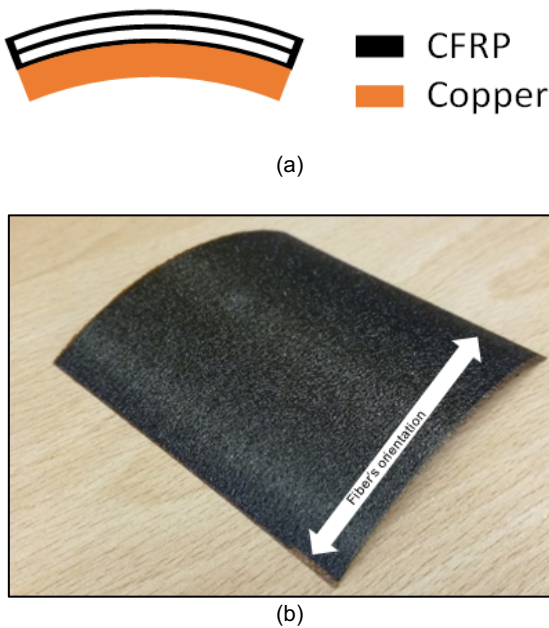
Figure 3. (a) Schematic showing the fibers' orientation in relation to the curvature. (b) Image of the curved Cu-CFRP combination where sample width is ~75mm.
