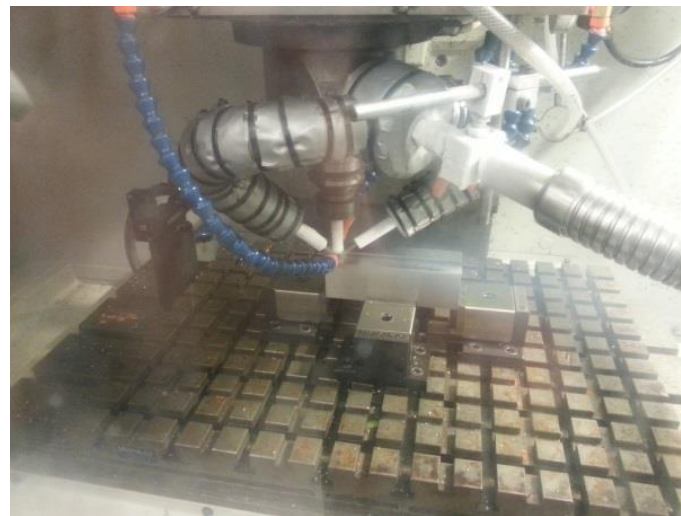
Figure 6, Pictorial view of the hybrid cryogenic MQL system
