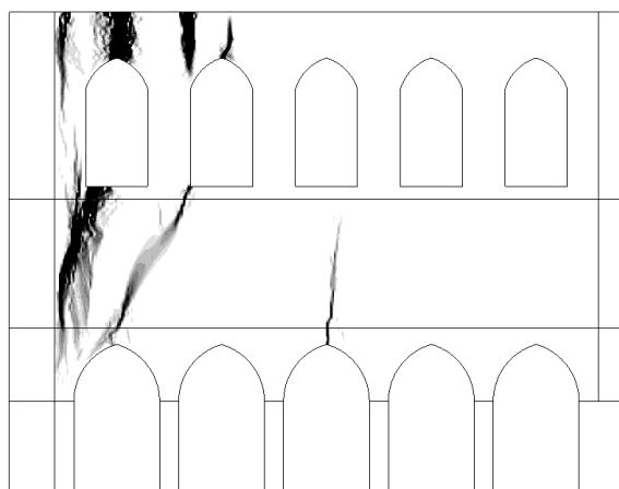
378 Figure 9 Crack patterns for application of load in single analysis phase.
