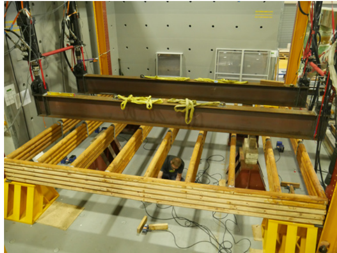
Figure 18: Prefabricated floor system using composite log wall elements consisting of profiled round small-diameter timbers and angled through-bolts for shear resistance (Thornton and Blair, 2014, 2016, Loggo, n.d.). Photograph courtesy of Loggo Pty Ltd.
