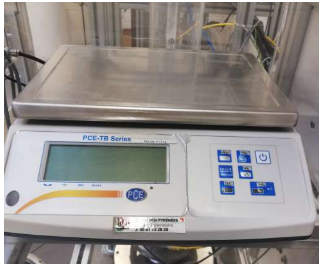
Figure 2.9: Balance for entrainment flux tracking
