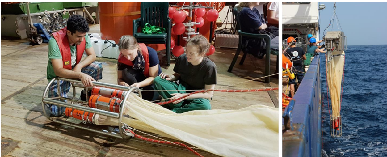
Figure 5.3.2: Preparation (left) and deployment (right) of the Hydrobios multinet with five nets for zooplankton sampling during METEOR cruise M160.
