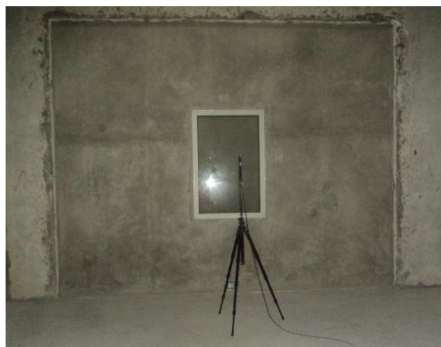
Fig. 2. Front view of composite wall specimen.
