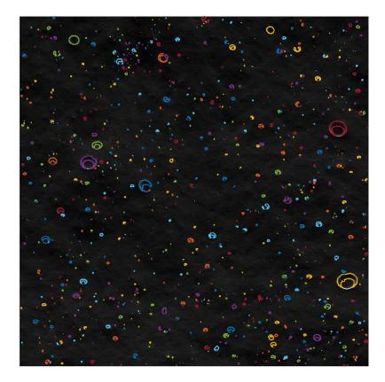
Figure 2.24: The same obstacle detection algorithm was run on this 1-m resolution elevation data from Shackleton crater on the Moon. The algorithm does a much better job in an environment with sharp, clearly-defined obstacles like micro-craters and boulders.
