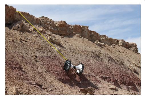
Figure 1.10: Axel rappelling down a rocky slope during a field test near Black Point Lava Flow in Arizona. The tether in this image is highlighted in yellow, for visibility.
