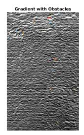
Figure 2.23: The gradient magnitude of the DEM on the left, with obstacles superimposed in color. This particular terrain seems composed of regular sandy dunes, so it is unsurprising that very few obstacles were detected.
