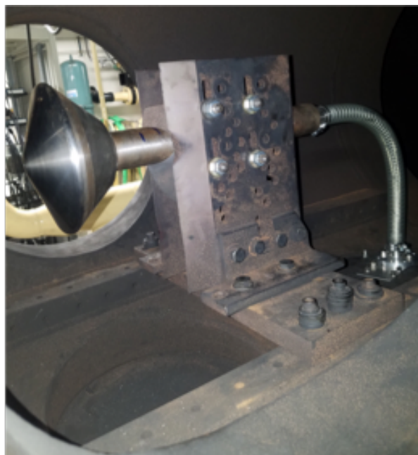
Figure 6.1: 7" diameter test article mounted at 0^\circ AOA in the T5 test section.
