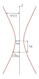
Figure 4.4. Schematic of a focused Gaussian beam used for modeling the exposure pattern in TPL
