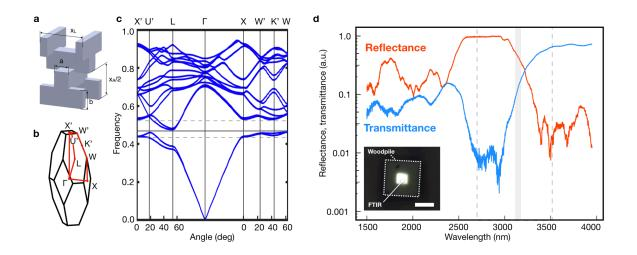
Figure 4.15. Optical characterization of 3D photonic crystals fabricated using the developed nanoscale AM process
