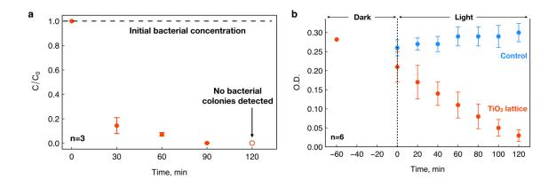
Figure 5.9. Proof-of-concept E. Coli and methylene blue (MB) experiments to evaluate photocatalytic activity of 3D micro-architected titanium dioxide.
