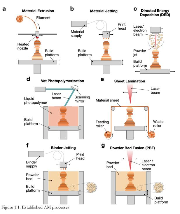
**a** Material Extrusion **b** Material Jetting **c** Directed Energy Deposition (DED) **d** Vat Photopolymerization **e** Sheet Lamination **f** Binder Jetting **g** Powder Bed Fusion (PBF)
