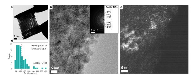
Figure 4.12. TEM characterization of as-fabricated  $TiO_2$  3D architectures.
