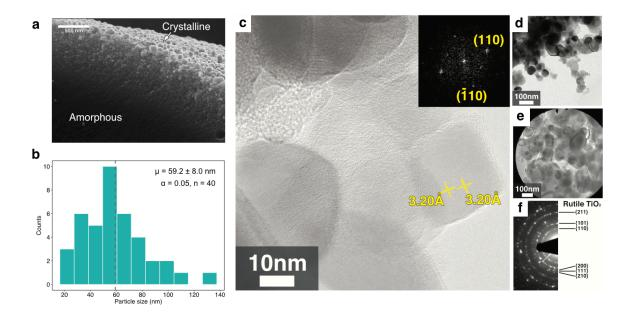
Figure 5.5. TEM and SEM characterization of printed titania structures.
