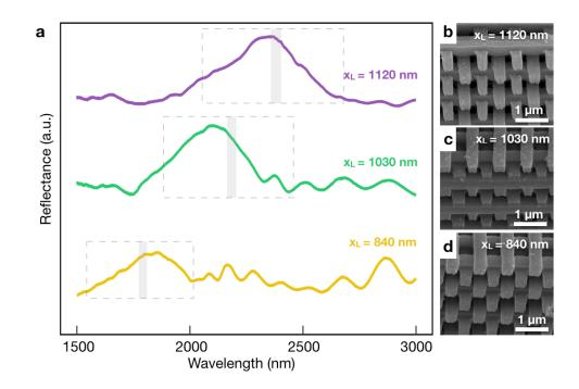
Figure 4.16. FTIR characterization of 3D woodpile architectures fabricated using a reduced precursor amount approach.
