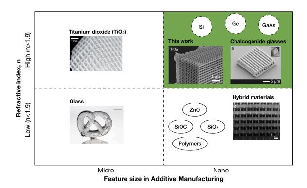
Figure 4.17. AM process landscape showing micro- and nanoscale AM processes of low- and high-refractive index materials
