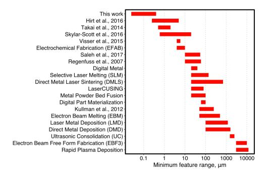
Figure 2.4. Comparison of minimum feature sizes for commercial and potentially scalable metal additive manufacturing technologies.
