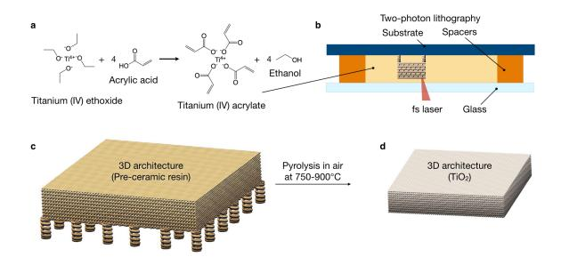
Figure 4.1. Process for nanoscale additive manufacturing (AM) of titanium dioxide
