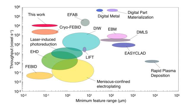
Figure 2.5. Throughput vs minimal feature range for established AM processes and emerging micro- and nanoscale metal AM.
