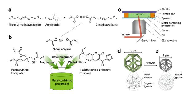
Figure 2.1. Process for nanoscale additive manufacturing of metals.
