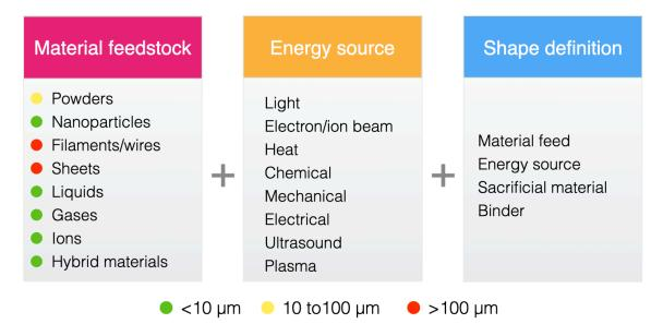
Figure 1.5. AM process framework showing the role of the material feedstock on the minimal feature size
