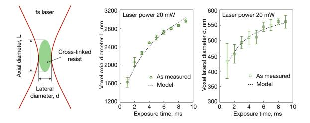
Figure 4.6. Predicted and measured voxel dimensions for the hybrid titania resist for a constant laser power of 20 mW as a function of the exposure time.
