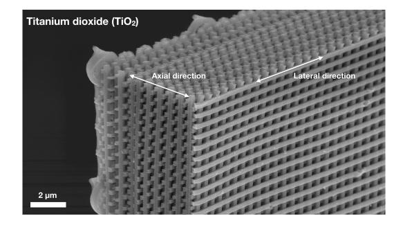
Figure 4.8. SEM image of as-fabricated woodpile FCT architecture showing lateral and axial directions within the crystal
