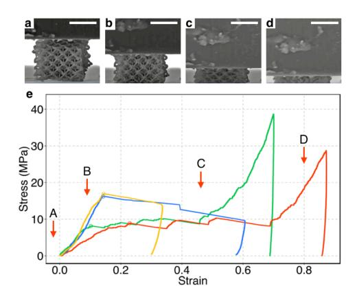
Figure 3.3. *In-situ* uniaxial compression of 3D printed nickel octet nanolattices.
