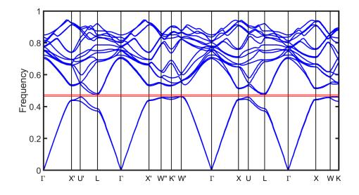
Figure 4.14. Band diagram from PWE showing the emergence of a full photonic bandgap in a simulated woodpile tetragonal architecture
