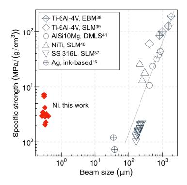
Figure 3.4. Specific strength-beam size plot showing properties of nickel nanolattices compared to other metal AM processes.
