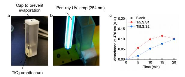
Figure 5.13. Experimental setup for photocatalytic characterization of 3D architected titanium dioxide
