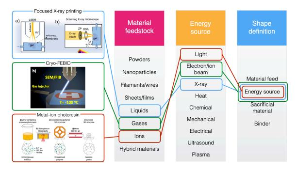
Figure 6.2. Recent nanoscale AM processes and how they fit into the AM process framework.
