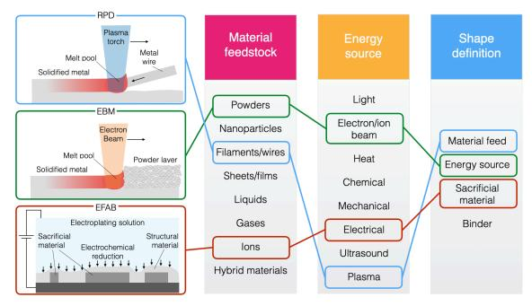
Figure 1.4. Example of using AM framework to analyze three established metal AM processes: RPD, EBM, and EFAB
