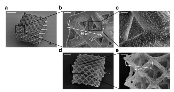
Figure 2.2. SEM characterization of the samples fabricated using nanoscale metal AM.
