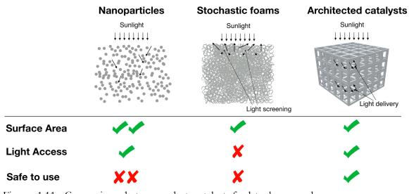
Figure 1.11. Comparison between photocatalyst feedstocks, namely nanoparticles, stochastic and deterministic foams, in terms of surface area, light access and safety
