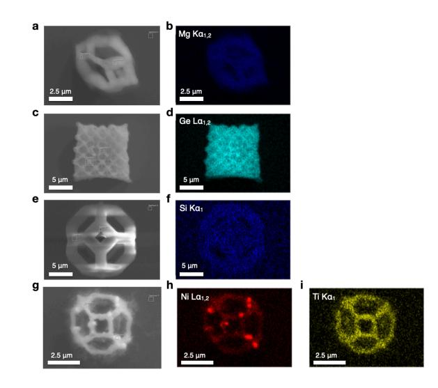
Figure 2.6. Extending the developed nanoscale AM process to incorporate other materials
