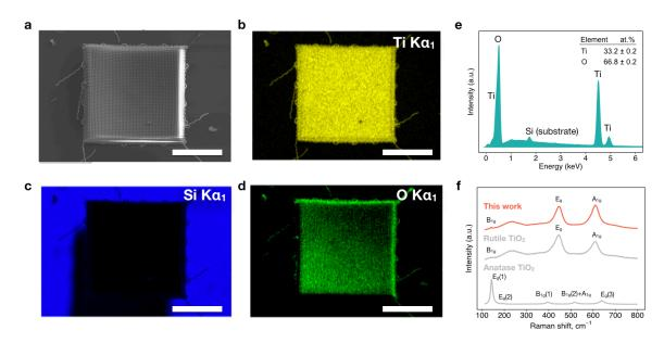
Figure 4.11. Characterization of chemical composition and phase of TiO<sub>2</sub> using SEM EDS and Raman spectroscopy.
