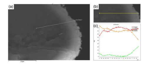
Figure 5.6. EDS characterization of a beam cross-section of a 3D printed titania octet lattice.
