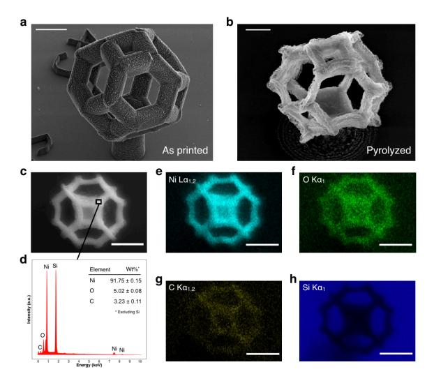
Figure 3.1. Energy Dispersive Spectroscopy (EDS) characterization of fabricated metal nanostructures.
