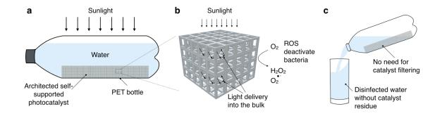
Figure 5.1. Concept of a household solar water disinfection device.
