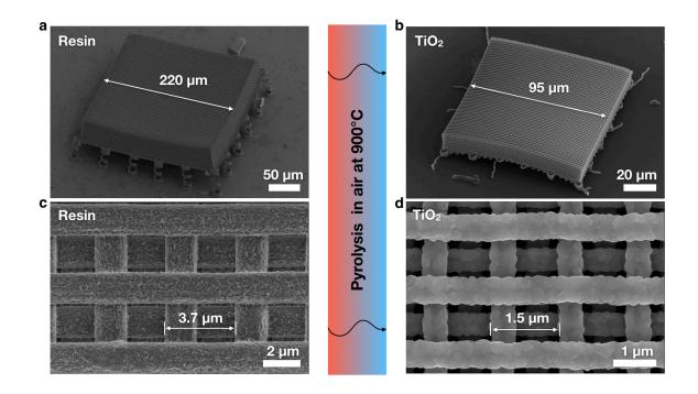
Figure 4.7. SEM characterization of as-fabricated TiO<sub>2</sub> 3D architectures.
