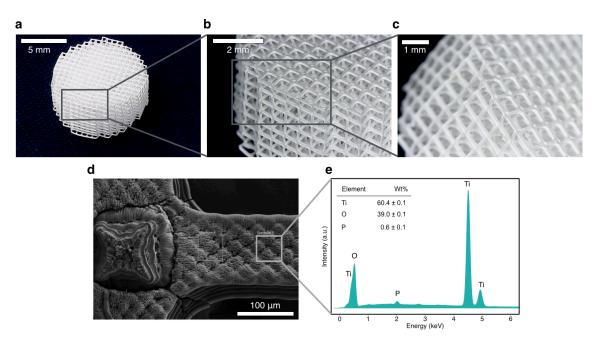
Figure 5.8. 3D printed titania cylinder comprised of simple cubic unit cells with unit cell dimensions of  $600 \,\mu\text{m}$  and beam diameters of  $150-200 \,\mu\text{m}$ .
