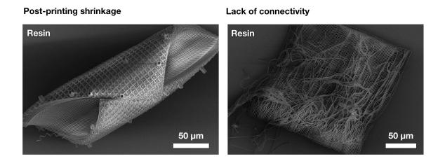
Figure 4.2. SEM images of TPL-fabricated resin 3D structures showing representative printing defects
