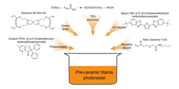
Figure 5.2. Pre-ceramic photopolymer formulation for SLA-based 3D printing of titanium dioxide
