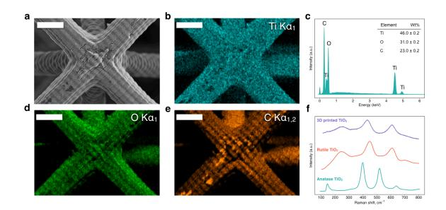
Figure 5.4. EDS and Raman characterization of printed titania structures.
