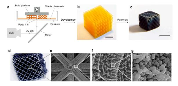
Figure 5.3. Process for AM of titania and SEM characterization of printed titania structures.
