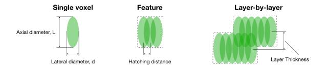
Figure 4.3. The importance of predicting the voxel size for control of feature dimensions in two-photon lithography
