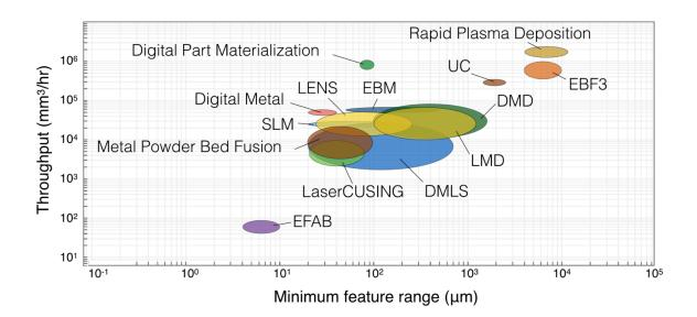
Figure 1.2. Resolution vs throughput for established metal AM processes
