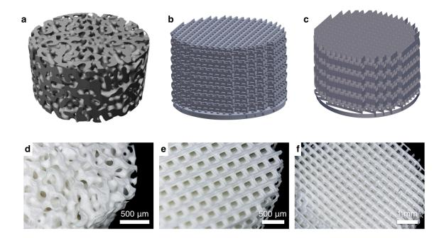
Figure 5.11. Stochastic and deterministic architectures fabricated for photocatalytic experiments
