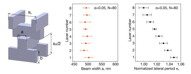
Figure 4.9. Beam widths and lateral periods in the axial direction of asfabricated titania woodpile as measured by SEM
