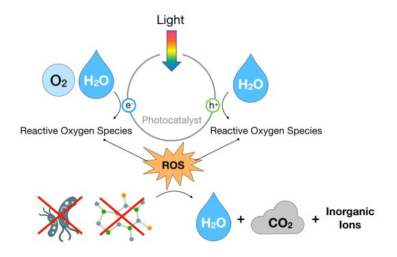
Figure 1.9. Photocatalytic generation of reactive oxygen species (ROS) for water treatment
