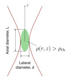
Figure 4.5. Modeling voxel dimensions using radical concentration profile within a focused Gaussian beam.
