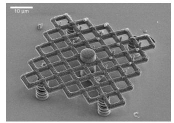
Figure 2.3. SEM image of a representative supporting structure used to decouple the part from the substrate during pyrolysis.
