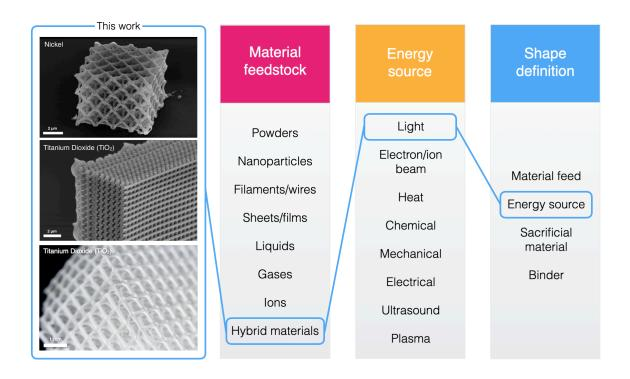
Figure 6.1. Nanoscale and microscale AM processes developed in this work and how they fit into the AM process framework
