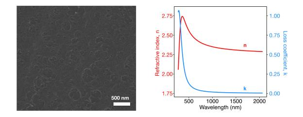
Figure 4.13. SEM image of a 100 nm-thick film of  $TiO_2$  on Si prepared for ellipsometry measurements and ellipsometry data for wavelengths between 275 nm and 2  $\mu$ m
