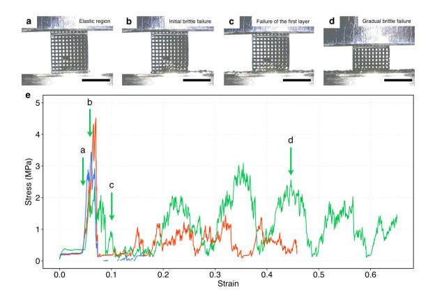
Figure 5.7. Uniaxial compression test of printed titania/carbon cubic lattices.
