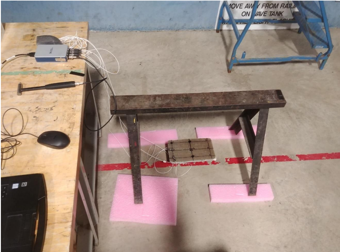
Figure 3.7: Experimental Setup for Composite Hull Plate
