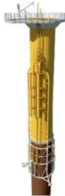
Sketch drawing of a monopile.
