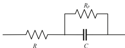
Figure 6. Classical equivalent circuit of a double layer capacitor showing its three basic characteristics: the internal resistance ( R ), its capacitance ( C ), and its self-discharge resistance ( R_p ).
