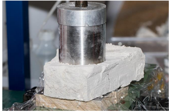
Figure 2 Pressing-out of block sample. The cylindrical ring is placed on top of the chalk ready to be pressed into the chalk by the hydraulic jack.
