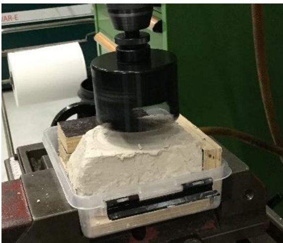
Figure 4 pressing-out in drilled core sample. A spoon bit is used to drill a core sample.
