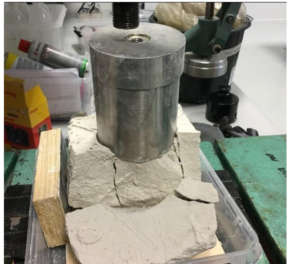
Figure 3 Pressing-out of block sample. The cylindrical ring has been jacket into the chalk, resulting in cracks in the chalk.
