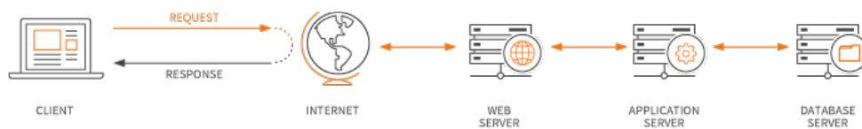
Figure 3.1: How a Web Application works (source: [24])
