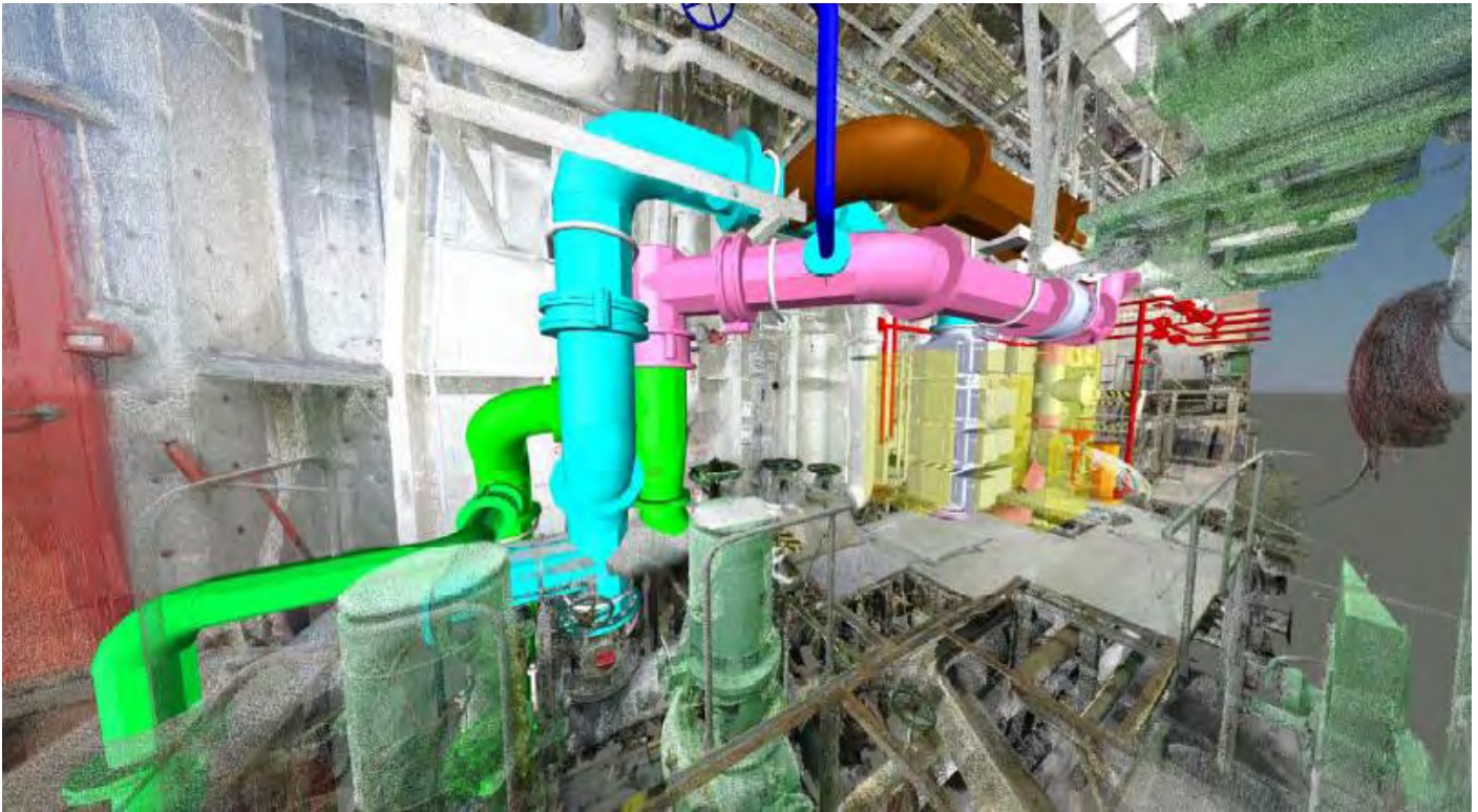
Figure 15 Design of a BWTS retrofit project on a bulk carrier. Source: Author
