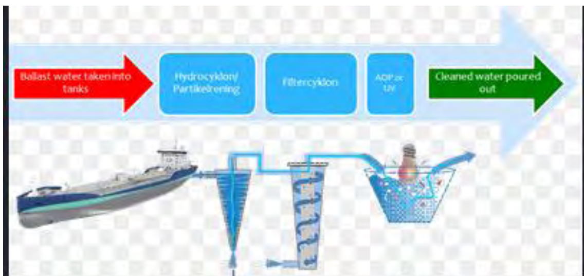
Figure 6 Hydro cyclone process. - Source: http://www.fonte.se/Ballast-water-treatment.html
