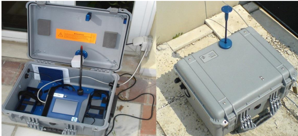
Figure 112 PM10 monitoring Instrument (Dusttrak 8530) placed inside its environmental enclosure.
