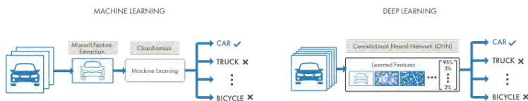
Figure 2.5: Comparing a machine learning approach to categorizing vehicles (left) with deep learning (right), source: mathworks.
