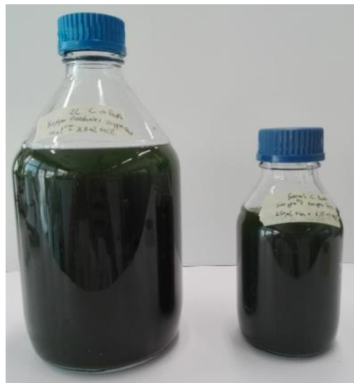
Figure 9 – Microalgae culture from A4F raceway for biopolymer and \text{FeCl}_3 flocculation test.
