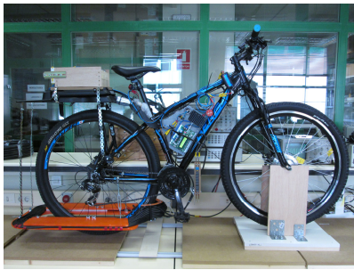
Figure 7. E-bike specially adapted with a pick-up coil and power circuitry, shown during workbench tests.
