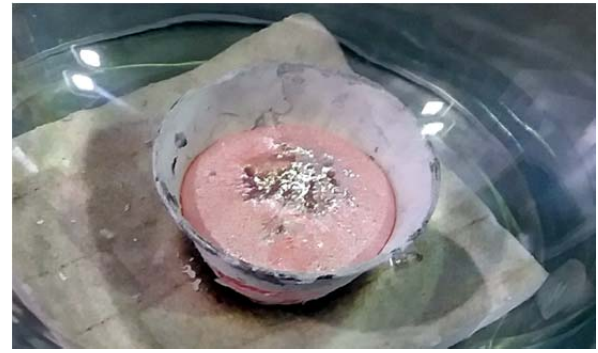
Fig. 3. RPT sample inside the vacuum chamber with bubbling hydrogen on the surface of the aluminium taken from the metal bath at 800°C
