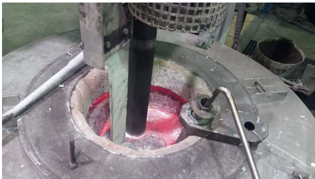
Fig. 2. Rotary degasser in the medium volume furnace
