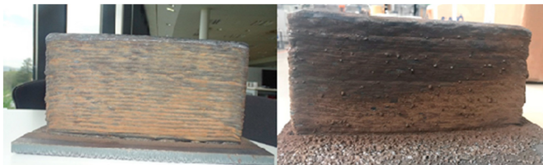
Fig. 1 (a) Test wall manufactured by PAW; (b) Test wall manufactured by GMAW.
