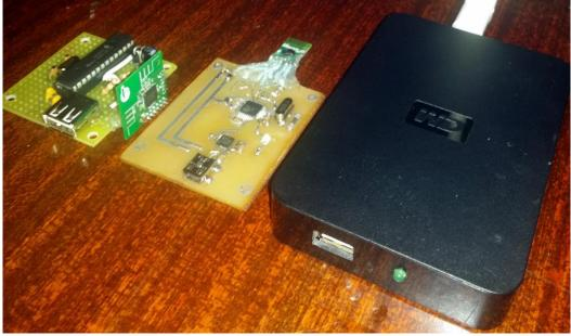
Spectrum Analyzer is a device for scanning and analyzing a specific frequency band, allowing you to detect and communicate wireless capabilities of
