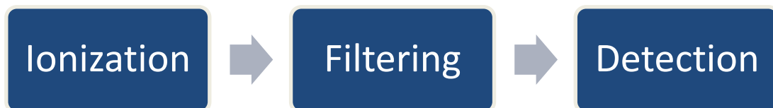
Figure 13. The operational principle of a residual gas analyser.
