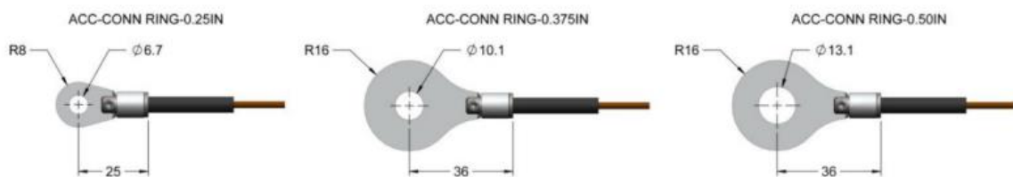
Figure 45 Rings lugs in 1/4, 3/8, and 1/2 sizes can be fastened to the end of the probes [48]
