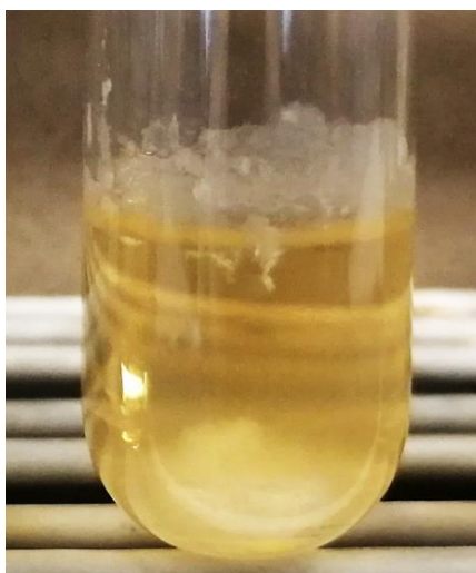
Figure 22. Bacterial growth on a PLA polished sample.
