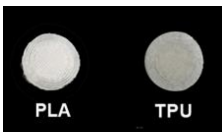
Figure 21. PLA and TPU 3D printed samples using the ironing feature.
