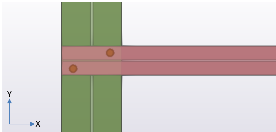
Figure 6. Bolts location of secondary beam (IPE160) for Beam 1-IPE360 /Beam 2-IPE160 (example)
