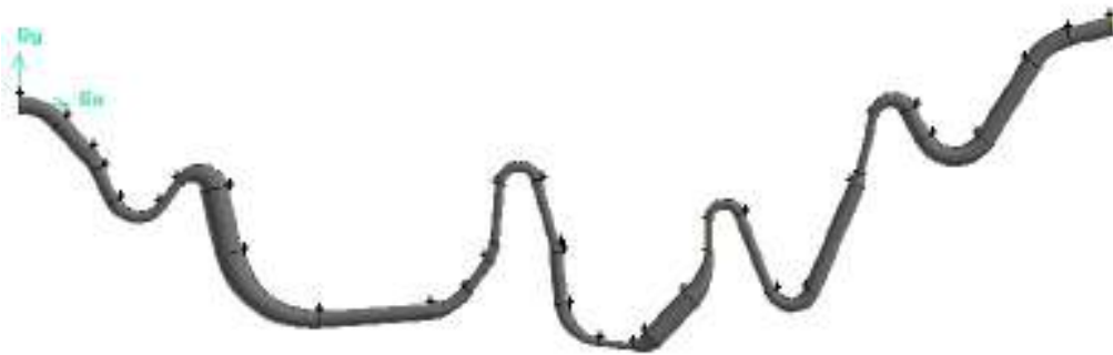
Figure 2. Pore space network created with the PMCFD model.
