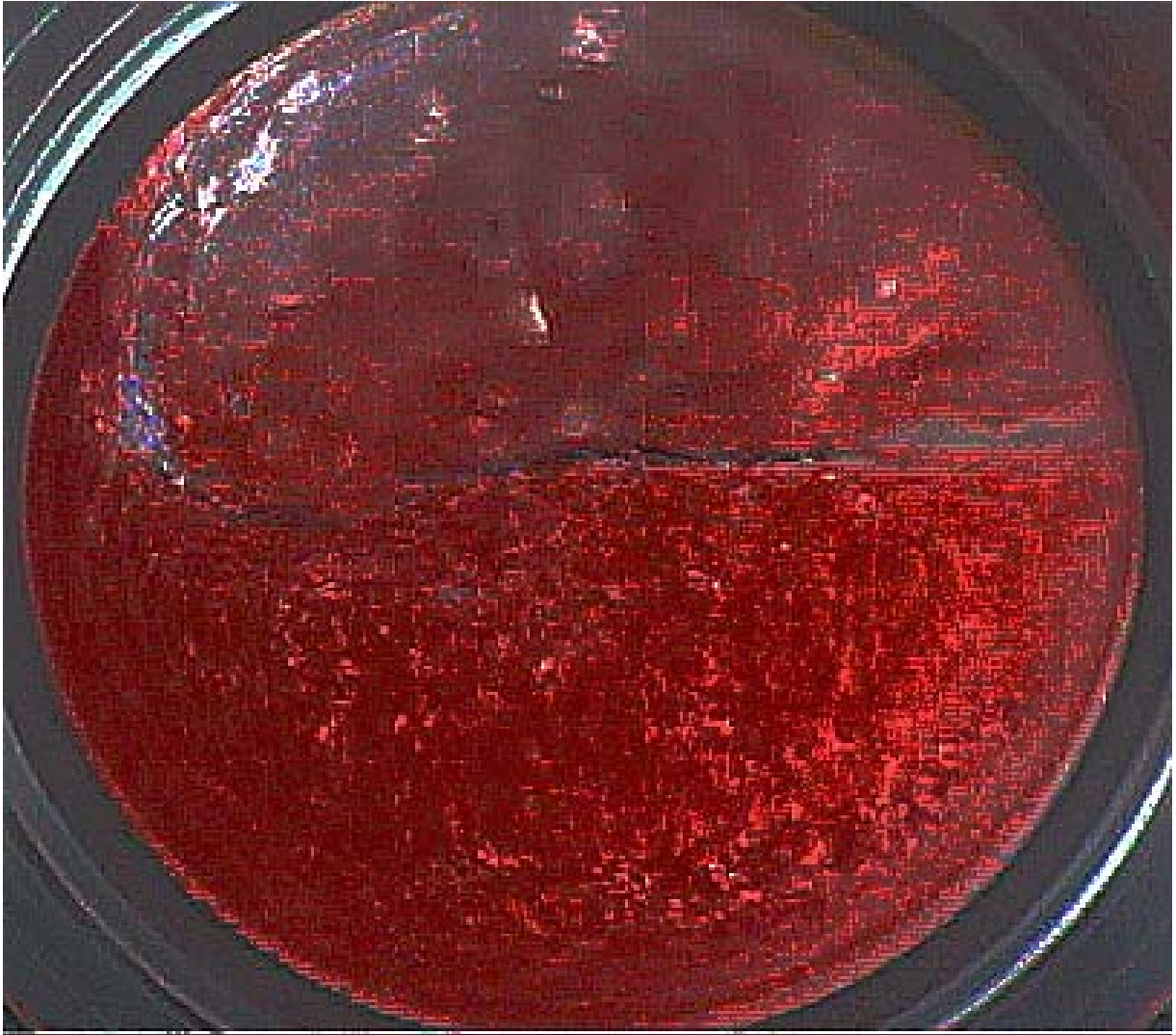
Figure 31. The standing pool of water over the narrow boundary layer, 7" cyl. 7/10 full, 320 RPM, (the picture is extracted from a video). The angular velocity is into the picture. The color scheme of the picture has been altered to improve visibility.
