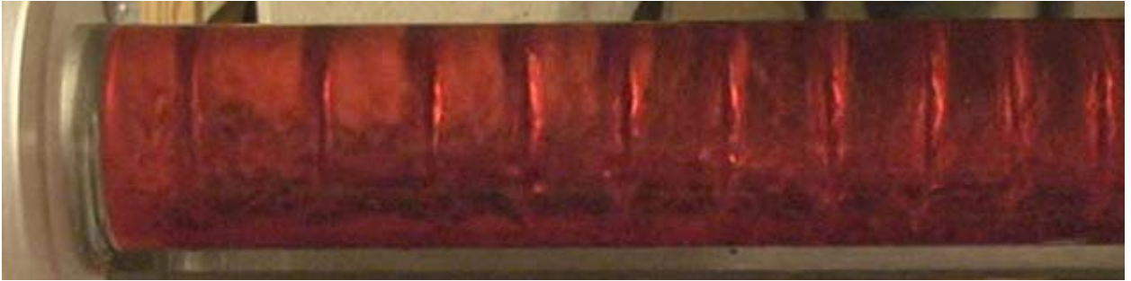
Figure 26 End view of the Gibbs phenomenon in a cylinder with an aspect ratio of \sim 10 , 5/10 fill-volume, (extracted from video).
