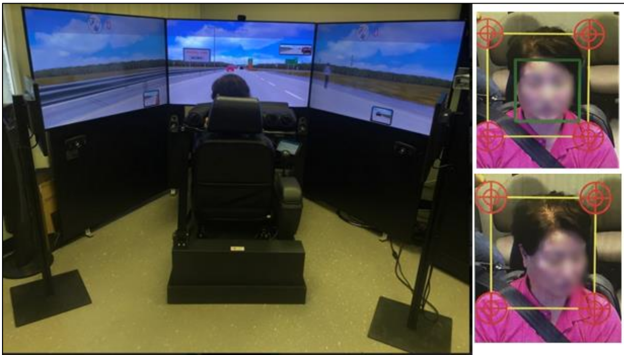
Figure 1. Driving simulator used for text reading and driving study
