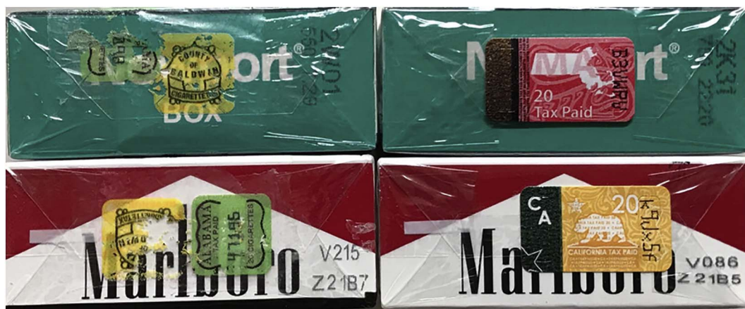
Fig. 1. Examples of damaged thermal (L) and undamaged encrypted (R) tax stamps.
