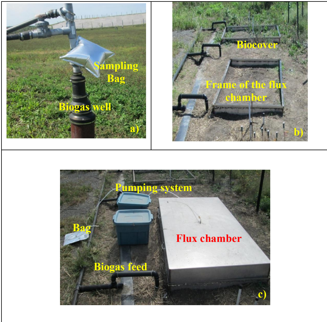
Fig. 2 Equipment to collect raw and emitted biogas a) Tedlar bags, b) metal frame, and c) flux chamber
