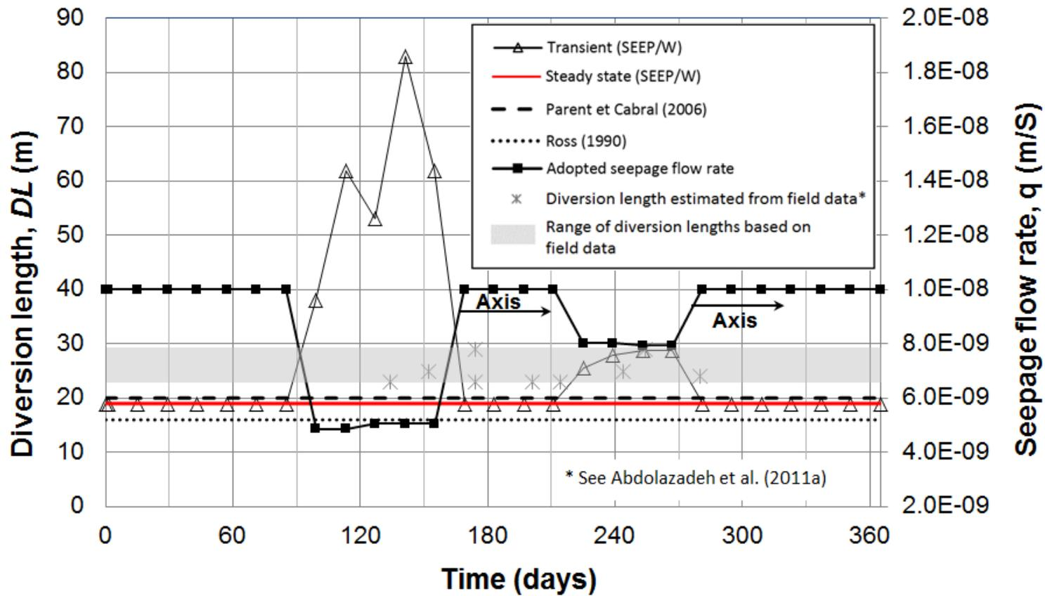
Figure 5: Evolution of the diversion length, as a function of the seepage flow rate (modified Visual HELP results, indicated as “adopted”; see Figure 4) and evolution of DL obtained by transient and, steady state analysis, as well as by using the Parent and Cabral (2006) and Ross (1990) models.
