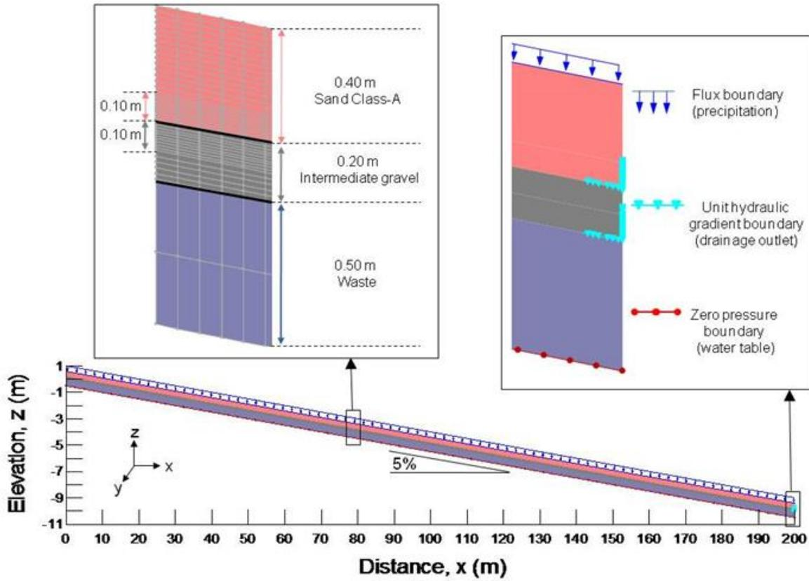
Figure 2: Basic model, geometry, dimensions, and boundary conditions of the Saint-Tite-des-Caps CCBE.
