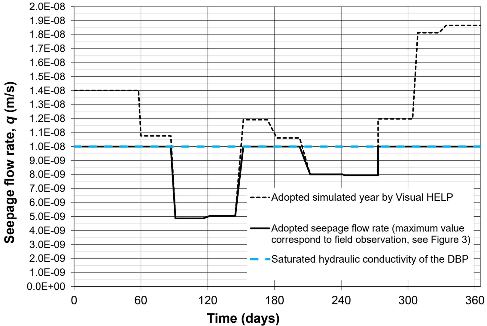
Figure 4: Visual HELP modeling results of the seepage flow rates through the DBP layer during a typical year.
