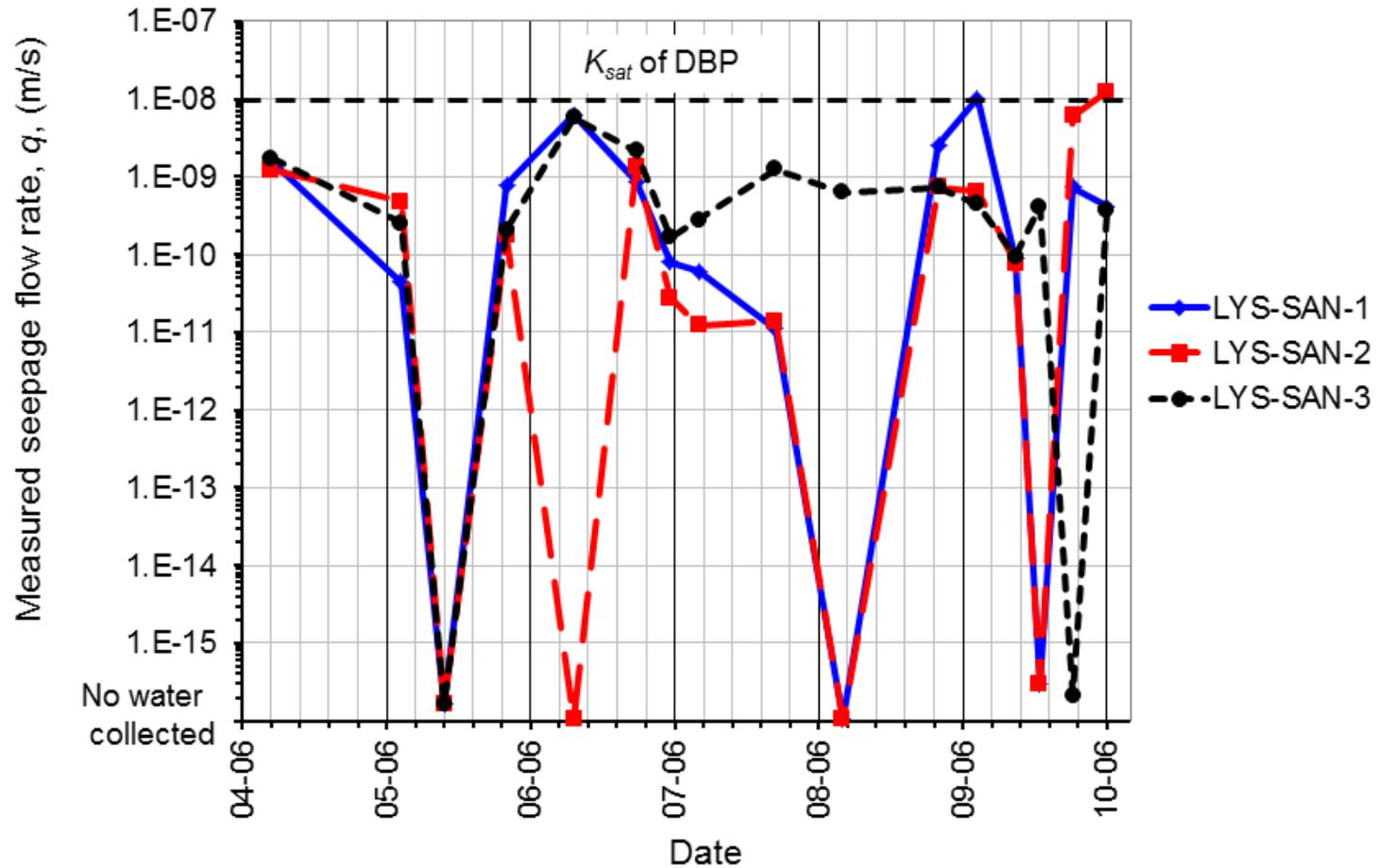
Figure 3: Evolution of seepage flow rates reaching the top of the sand/gravel capillary barrier by lysimeters installed in the sand layer at the Saint-Tite-des-Caps experimental CCBE, for year 2006 (adapted from Abdolhazadeh et al., 2008).
