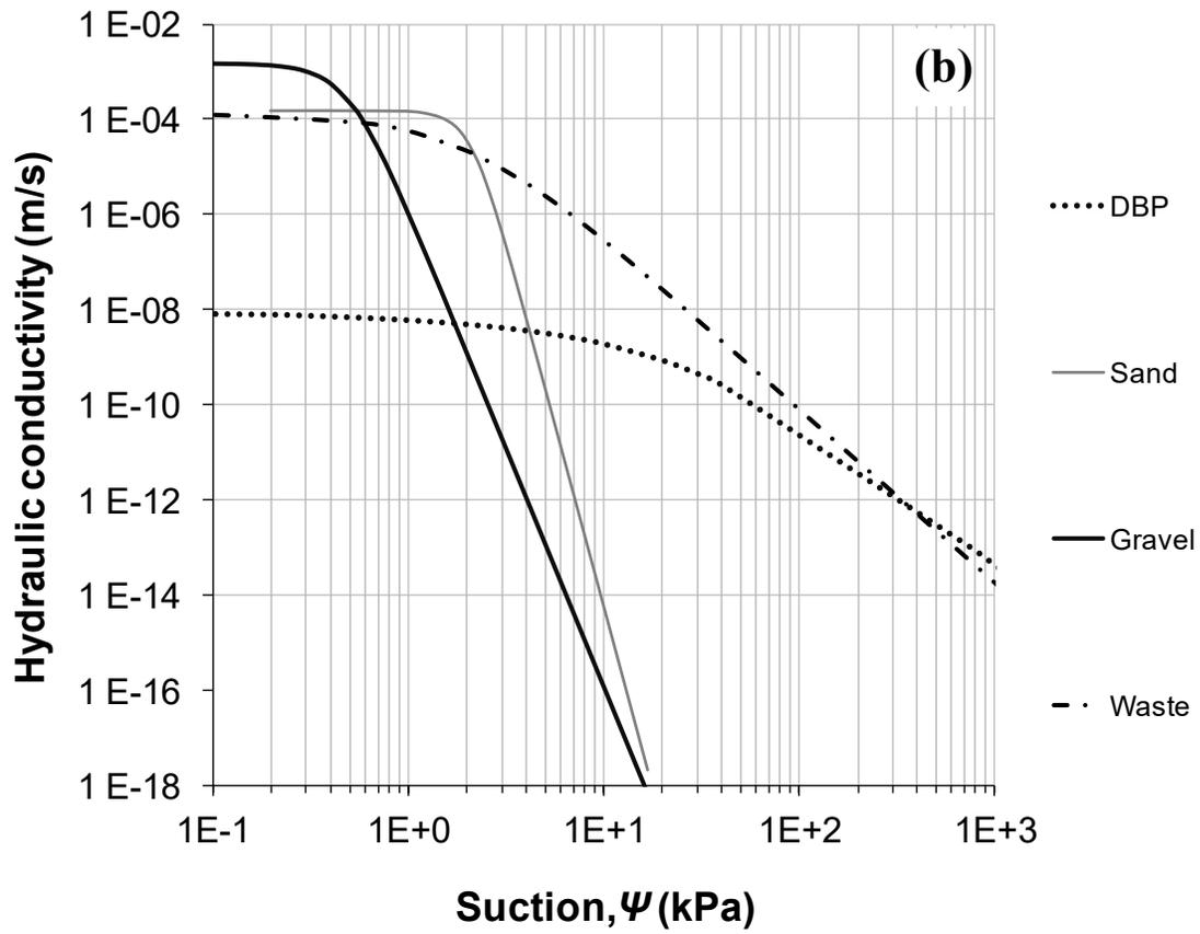
Figure 1: a) Water retention curve (WRC); and b)  $k_{fct}$  of the materials used in numerical simulations.
