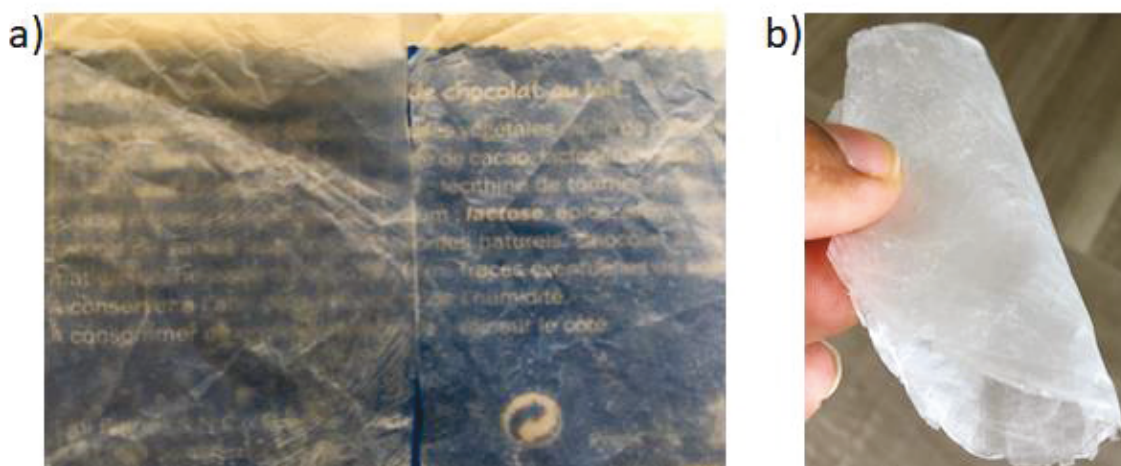
Figure 4. 3 a) The physical appearance of non-oxidized and oxidized TiO 2 coated films (from left to right respectively) b) flexibility of the film after coating
