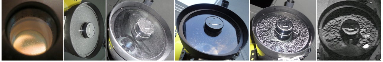
Figure 14: Left, photometer entry window: oil condensed on entry window. Next pictures, telescope entry window: rime icing (frost) and various deposition levels of precipitating ice crystals. Last one: after 2 h of clear sky snow.
