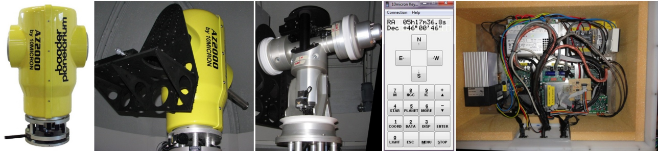
Figure 11: The AZ2000 star pointing mount in Eureka: with and without the insulating cover; virtual keypad; inside the mount/dome electronic box.
