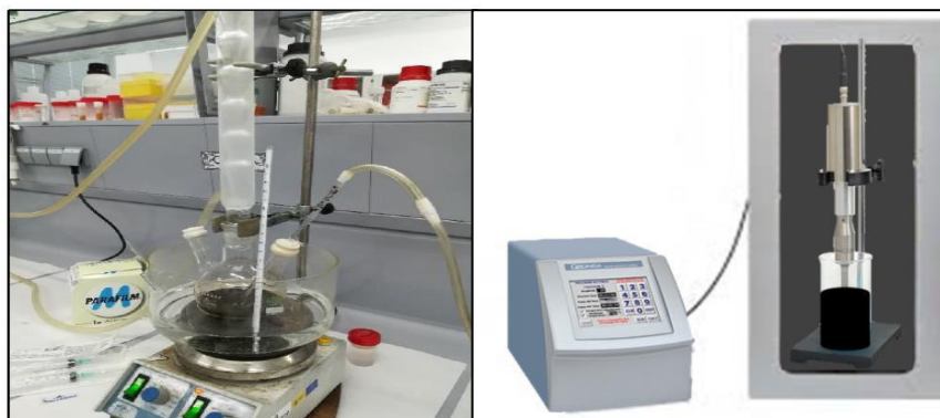
Figure 19. Simple comparison between a traditional co-precipitation method (left picture) and co-precipitation assisted by high power ultrasound (right picture)
