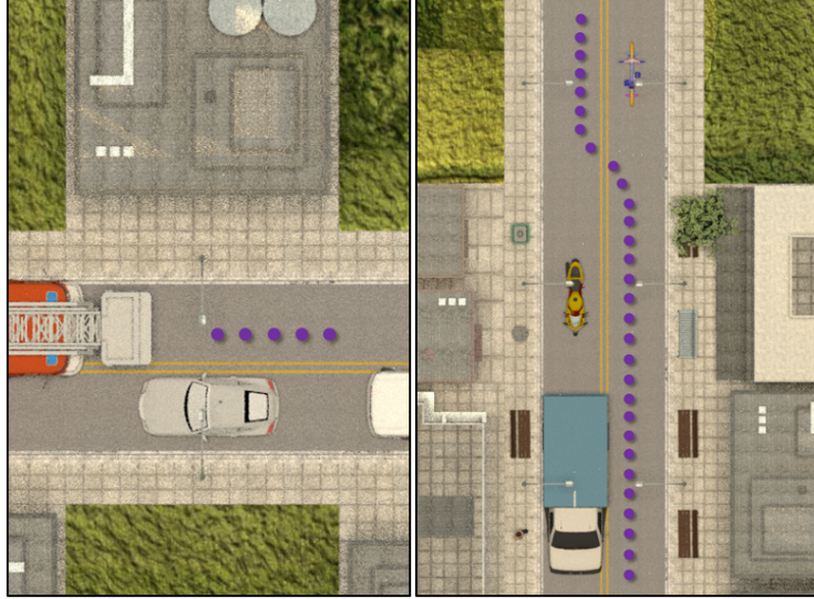
Figure 3.5: Two example sequences of capture locations. The sequence on the left contains 5 contiguous locations, and the sequence on the right contains 30. At each purple dot will be the set of four SV fisheye cameras to capture the scene from that location. Above each purple dot will also be a rectilinear camera to capture a true virtual top-view image.
