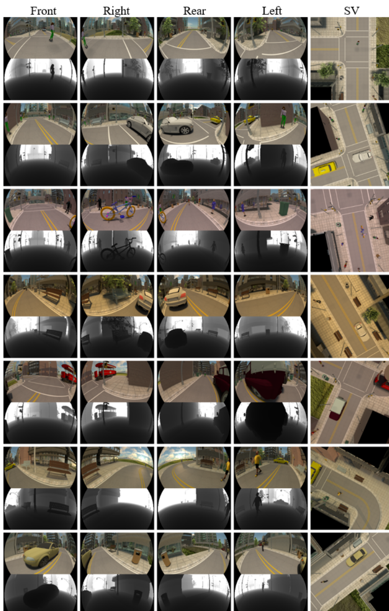
Figure 3.7: Example scenes from the database. Each set of images includes four fisheye images, their corresponding depth maps, and a true birdseye view capture. Note: for display, only depths < 25 meters are shown.
