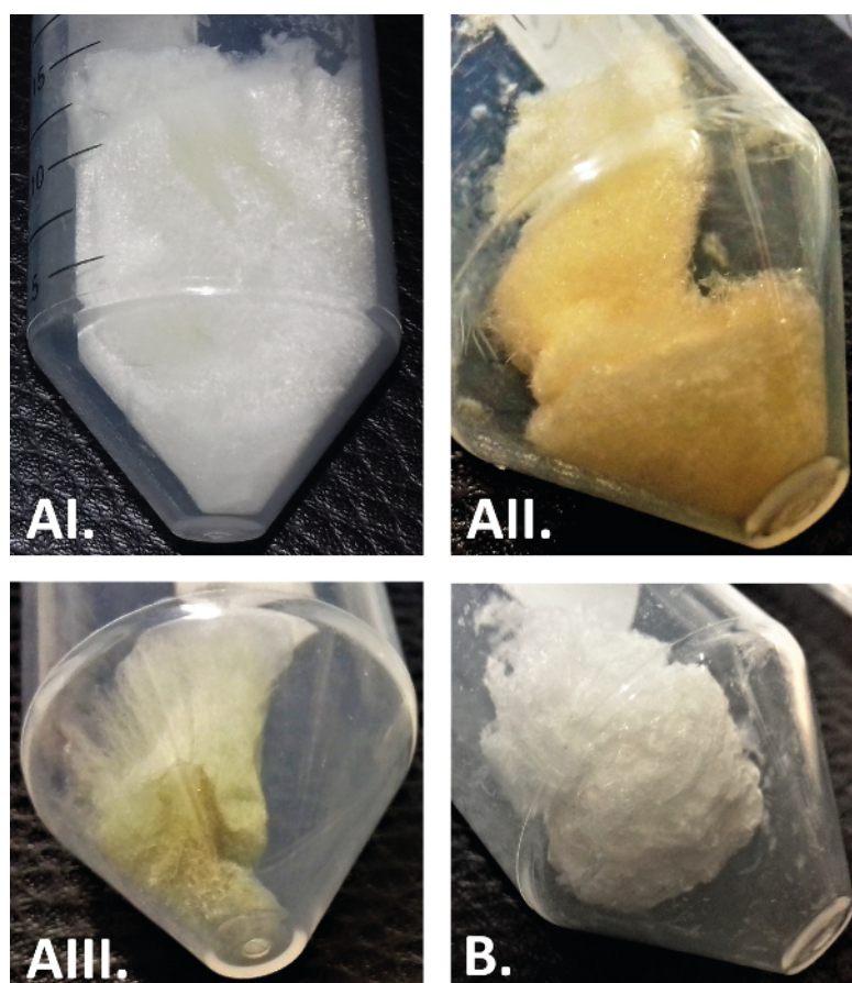
Figure 3: Lyophilized cyanobacterial polymers. (A) Three independent batches of polymers isolated from Synechocystis sp. PCC 6803: without visible contamination (AI), and with pigmentation indicative of contamination with carotenoids (AII) or cell debris (AIII). (B) Lyophilized polymer from Cyanothece sp. CCY 0110. Please click here to view a larger version of this figure.
