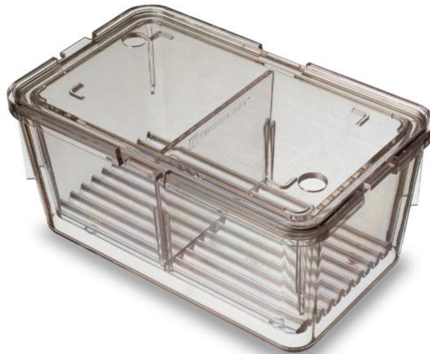
Figure appendix 4 Apparatus of zebrafish breeding tank. Prior to microinjection procedure, 1L external tank containing an internal tank with a perforated bottom, a device and a lid was seated with water facility system. After the spawning, animals were placed on other external tank using the internal tank and the fertilized eggs were easily collected from the bottom of the external tank. Adapted from Techniplast.
