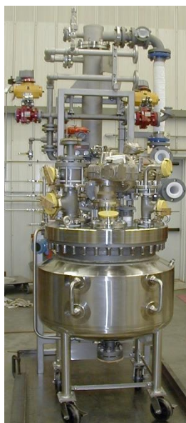
Figure 2.5. Agitated batch pilot plant crystallizer [41].
