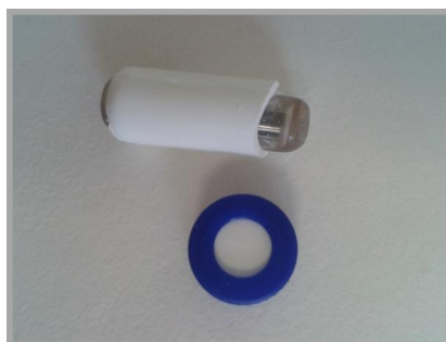
Figure 2. Magnetic molecularly imprinted stir bar (MMISB) developed for the extraction of patulin; a screw cap was placed below the stir-bar to illustrate its size (Reproduced with permission from [11]. MDPI under CC BY 4.0 , 2015).
