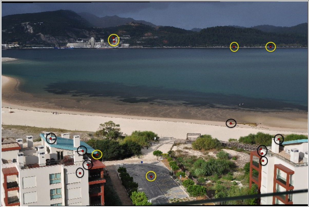
Fig. 7 OTP2 image overlapped to the reference (OTP5) using 15 pixels as references (red points with yellow/black circles).
