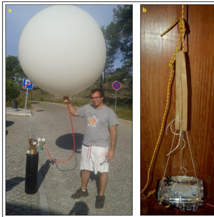
Fig. 5 Balloon filling process (a) and camera with waterproof case and tether system (b).
