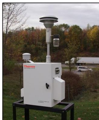
Figura 2.12 – Partisol-FRM Model 2000 Air Sampler (LSA, 2015).
