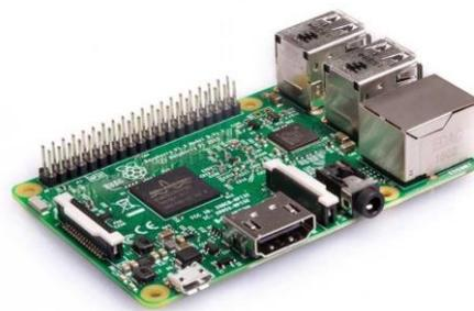
Fig 3.2 Raspberry Pi 3 Model B [18]
