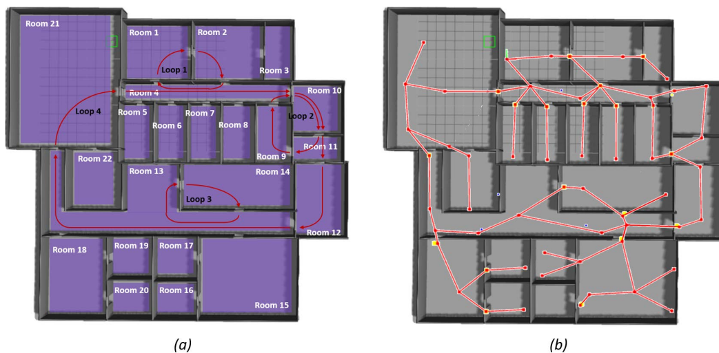
Figure 12. Results for the second big office simulated environment: (a) the environment and the different rooms and loops are indicated; and (b) the resulting topological map. The topological map is layered on top of the simulated environment in order to facilitate reader's comprehension.
