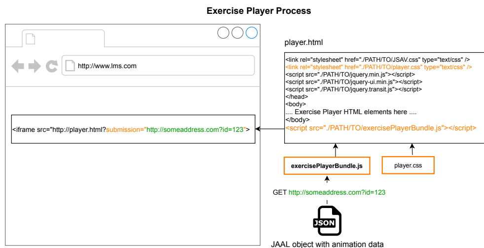
Figure 4.10. The Exercise Player component integrated into the LMS to replay the animation.
