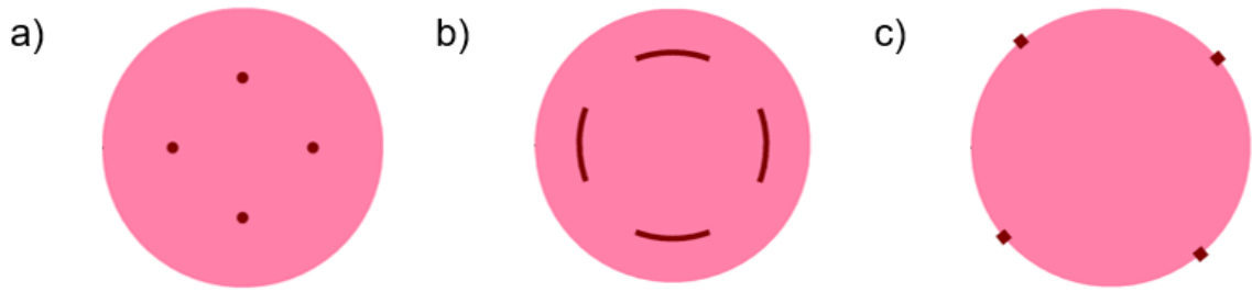
Figure 3.9: Via opening patterns used for the \text{XeF}_2 release. a) Circular-shaped via for top release. b) Arc-shaped via for top release. c) Square-shaped via for side release.
