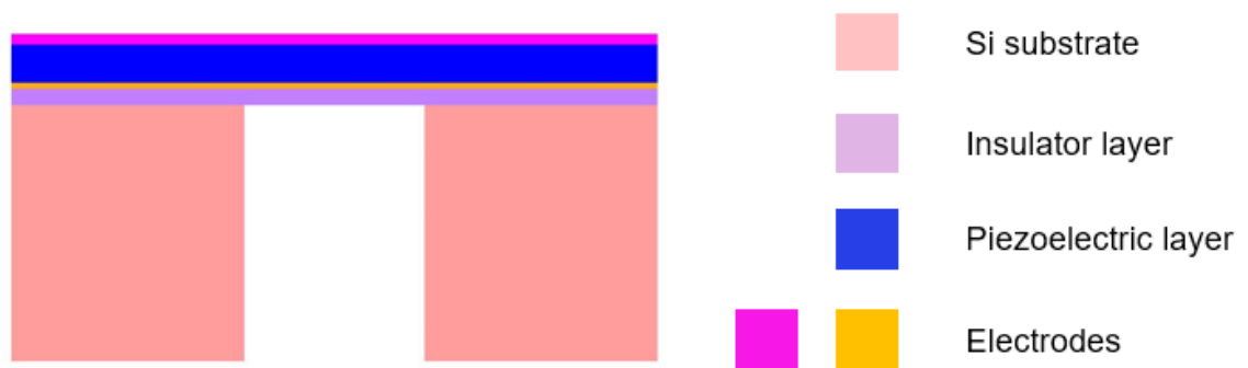
Figure 2.3: Schematic of a PMUT structure in which the diaphragm was defined by etching the back-side of the wafer. The vertical walls are obtained by DRIE etching.
