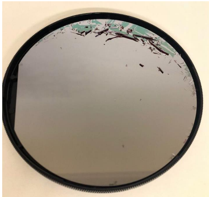
Figure 4.1: Sample wafer with annealed PECVD a-Si film. The a-Si was deposited on top of SiO 2 using PECVD at 300 °C and then annealed at 450 °C for 60 minutes.
