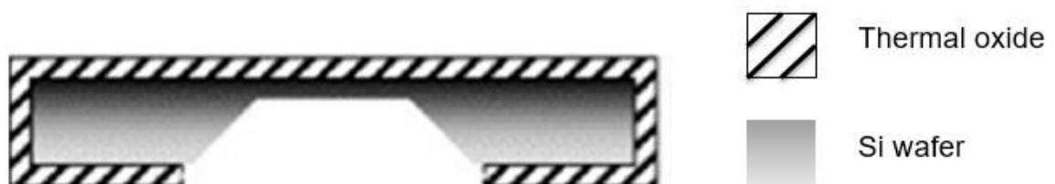
Figure 2.4: Schematic of a PMUT structure in which the diaphragm was defined by etching the back side of the wafer. The side-walls profile in the image are obtained by anisotropic wet etching. Image taken from: [2]
