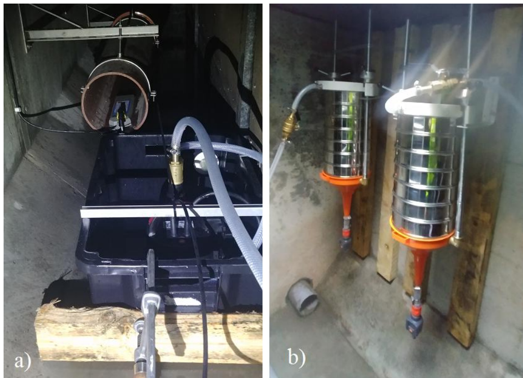
Figure 15. (A) Sampling pool attached next to the stormwater influent pipe in the filtration system and (B) sieve columns attached to the concrete wall of the underground sampling base.
