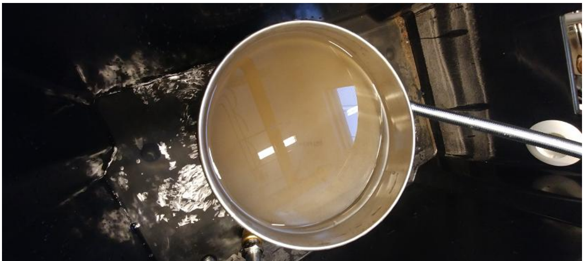
Figure 13. Clogged sieve due to solids ( \varnothing 20 cm) with a mesh size of 20 \mu\text{m}
