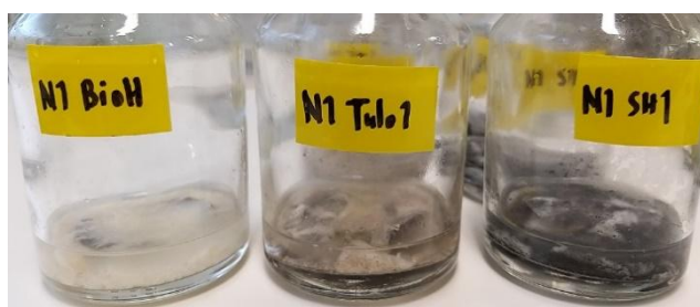
Figure 17. Coagulant on the bottom of sample glasses (Event 1).
