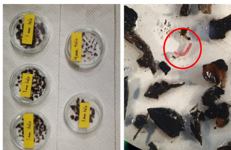
Figure 19. (A) Influent stormwater runoff solids ( 1000\text{-}5000 \mu\text{m} ) on Petri dishes and (B) a potential microplastic particle under stereomicroscope.
