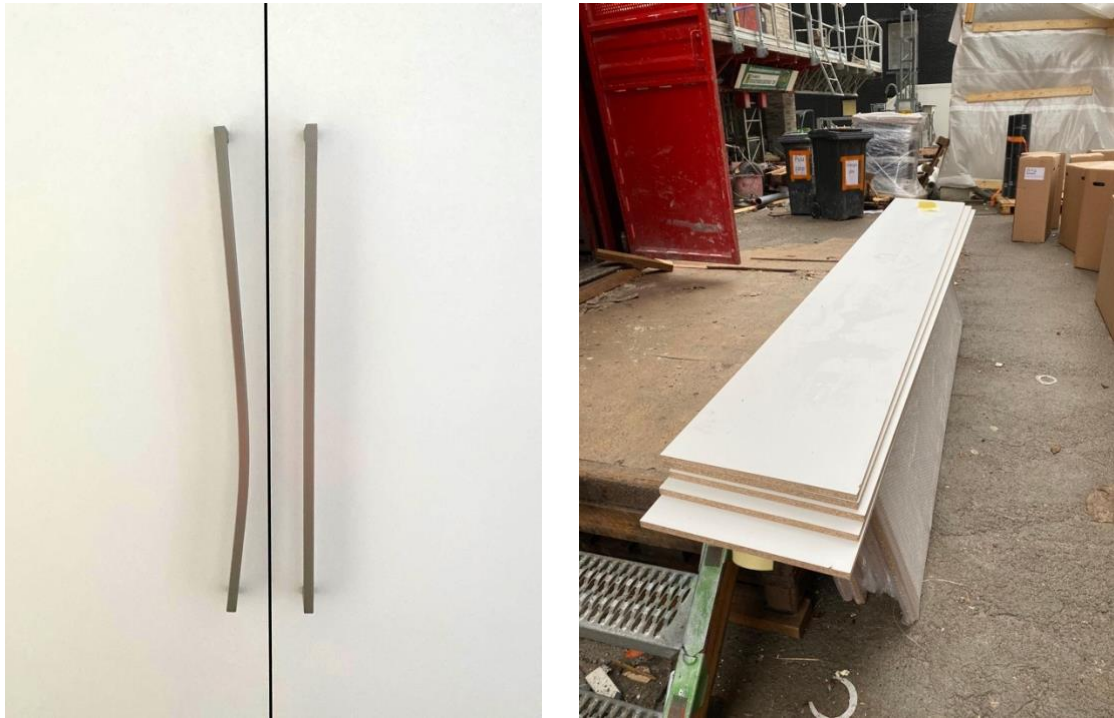
Figure 18. Mishandling of furnishing parts by the transportation company.
